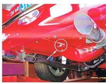
If you look under the trunk floor of your Sunbeam, you will see two metal guards welded to the floor to protect the fuel line. These guards are separated by a notch in the middle of the floor. It's an ideal place for a valve and is within easy reach from the rear of the vehicle.
